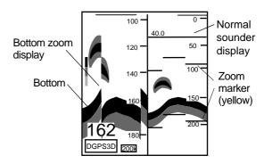
Figure 2-8 Bottom-zoom display plus normal sounder display
